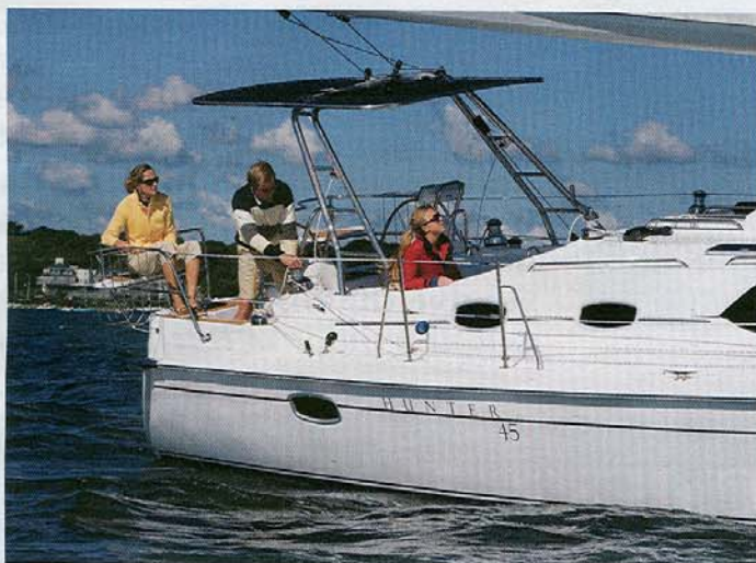
Hunter's trademark arch incorporating the traveler and the bimini keep the cockpit free of clutter.
